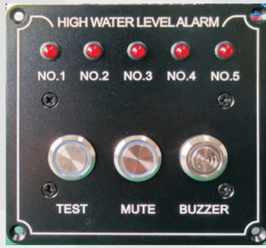
5-way high water level indicator alarm board
